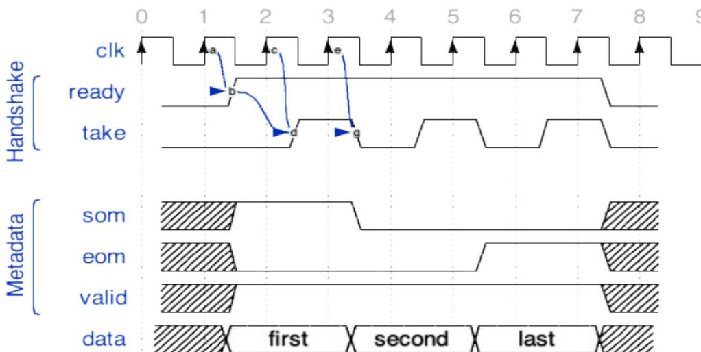
Figure 5: 3 word input message with worker adding delay
