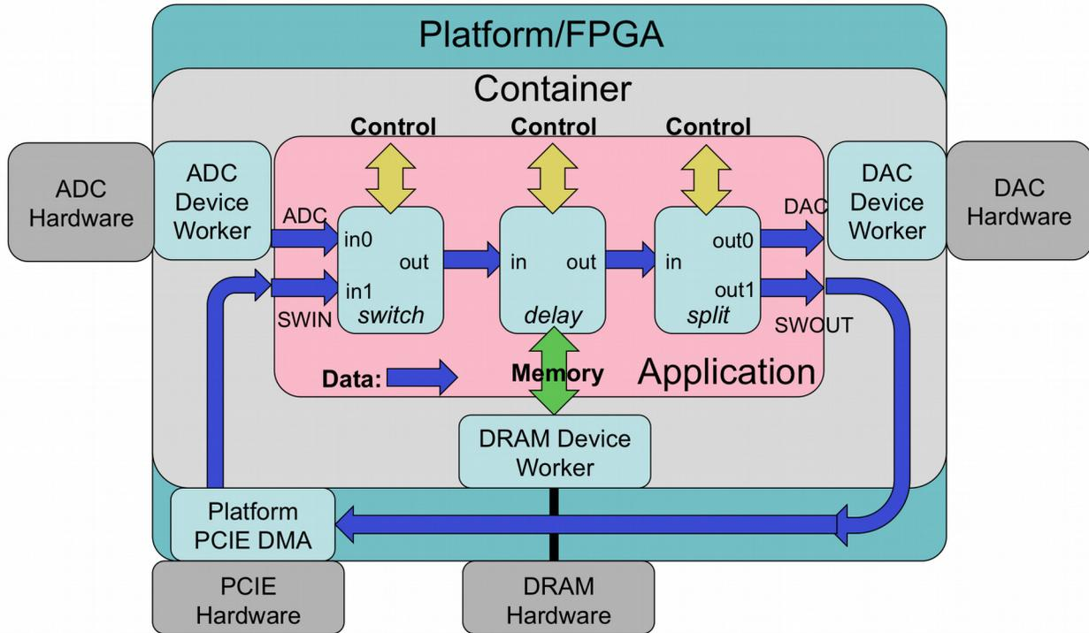
Figure 6: OpenCPI HDL Assembly on Container and Platform
