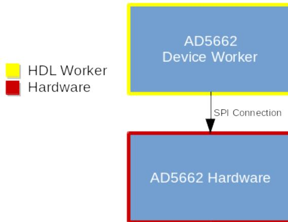
Figure 1: Top level block diagram of the e3xx\_mimo\_xcvr\_ad5662 device worker and hardware
