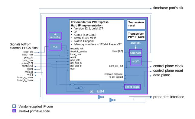
Figure 1: alst4 Functional Diagram
