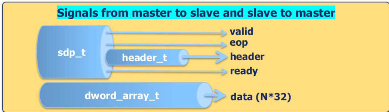
Figure 2: sdp_t Record Structure
