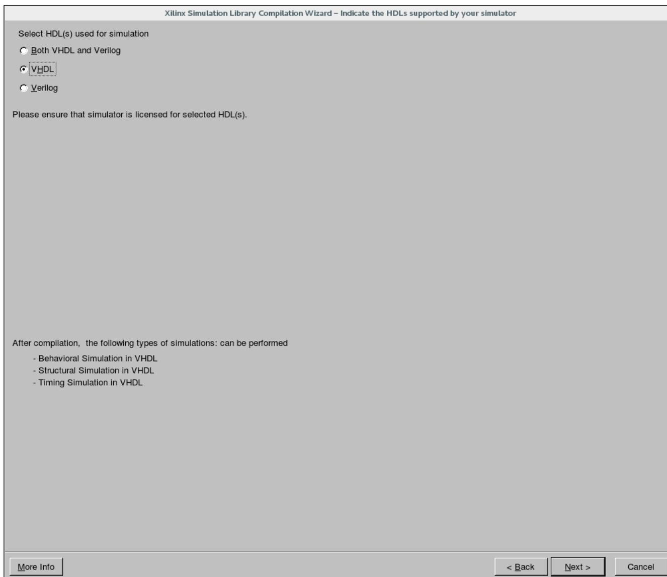
Figure 24: Compilation Wizard - HDLs to support simulator
